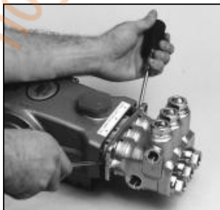
Removal of Manifold Head from Crankcase
